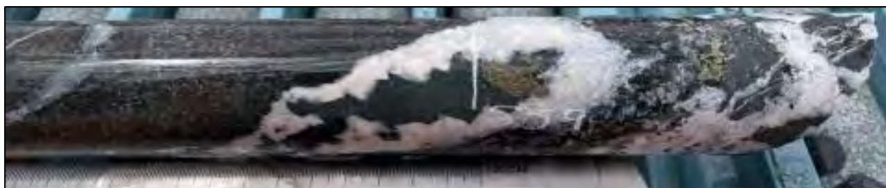
Figure 30: GDRCD007 – 559 m Example of a quartz-calcite vein in altered diorite with pyrite± chalcopyrite, chlorite "jigsaw" infill and minor brecciation. Source: Artemis.
