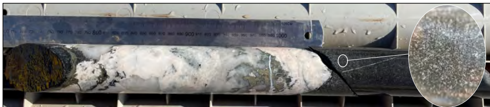
Figure 8: GDRCD007 – 538m, example of quartz-calcite vein in altered diorite with abundant pyrite± chalcopyrite-chlorite-actinolite infill. Close up example of disseminated inter-matrix sulphides in altered diorite.
