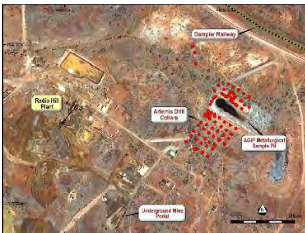
Figure 6: Radio Hill Mine area, processing plant and resource drilling location
